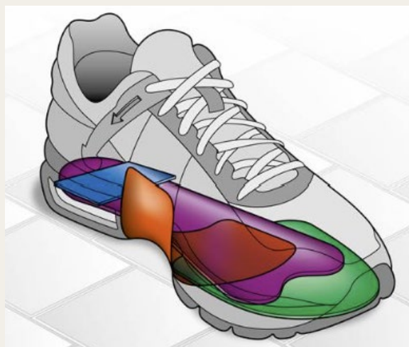
Figure 14: Schematic of a shoe with different areas where carbon plates could be beneficial. Image from Toray. 9
